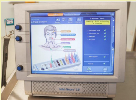
Figure 7: Facial nerve Monitoring Device, help surgeons to locate, monitor and identify the nerve. Also confirm nerve integrity at the end of surgery
