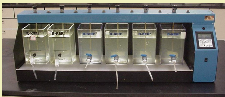
Figure 1: Installation of trial coagulation "Drop."
